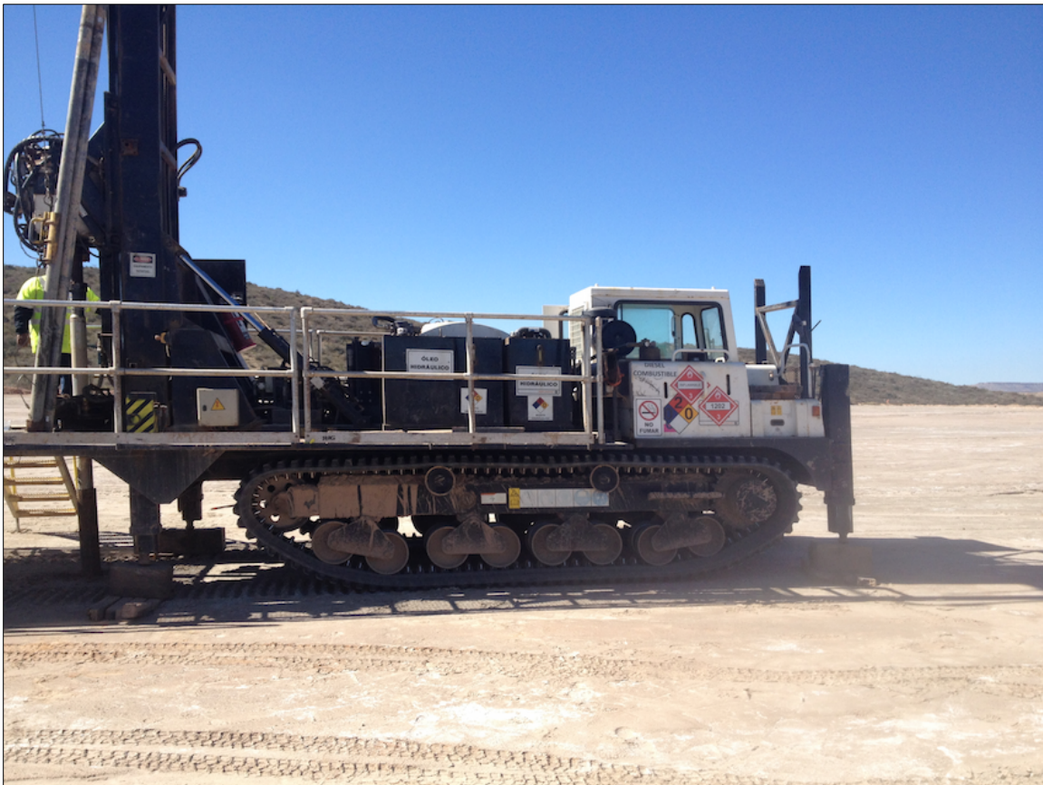
Figure 10.1 Track Mounted Sonic Drill Rig
