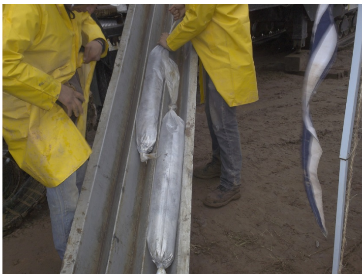
Figure 11.2 Esmeralda Tailings Sonic Drill Core Sampling
